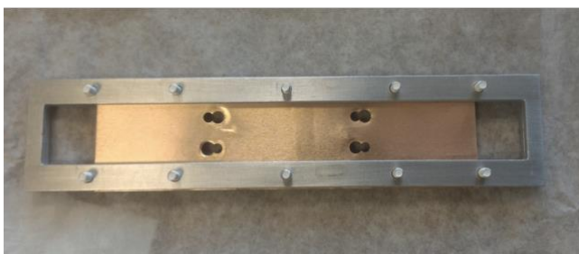
Figure 5: Slab placed in the frame for the deposition.
